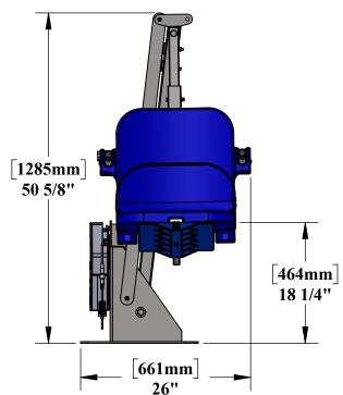
\*MEASUREMENT TAKEN WITH THE LIFT AT FULL LOAD
